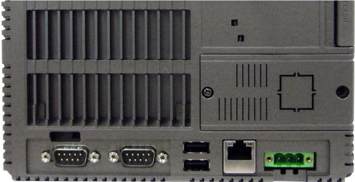
**Figure 4– I/O Port Arrangements for 6.5' TPC**
